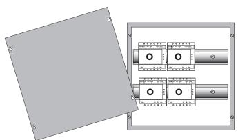
Includes two rows of DIN rail for mounting up to 6 ELCU-100s
