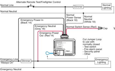
When wired as a shunt, the switching line is not used.
