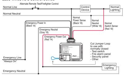
You can connect as many NC contacts (including EMTS-100) in series on the jumper loop wire as you want to a single ELCU. You cannot connect the NC devices in any other manner.
