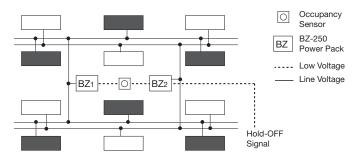
The occupancy sensor normally keeps lights On when the space is occupied. When a load shed command is received (from utility meter, BAS, etc.), lights connected to  $BZ_2$  are held Off. Remaining lights (connected to BZ) are still controlled by occupancy.
