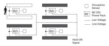
During store hours, a signal from a time clock to the BZ-250 holds lights On, regardless of occupancy. After hours, the clock schedule cancels the Hold-On and occupancy sensor control takes over.
