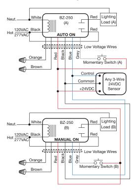
Connect two low-voltage switches, a ceiling sensor and two BZ-250s (one set to Auto-On and one set to Manual-On) for bi-level switching with manual-on operation.
