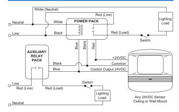
All Watt Stopper power packs should be installed in accordance with state, local, and national electrical codes and requirements. Power packs are designed to attach to existing or new electrical enclosures with 1/2 inch knockouts. (Check electrical codes in your area.) Most applications require UL listed, 18-22 AWG, 3-conductor, Class 2 cable for low voltage wiring. For plenum return ceilings use UL listed plenumapproved cables.
