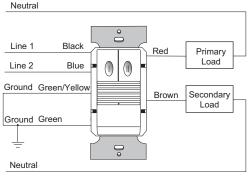
Two circuit wiring
