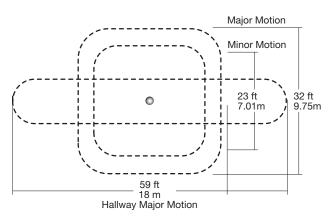
For optimal sensing of large spaces, place sensors so that coverage overlaps.
