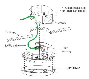
Mount to a 4" octagonal box (as shown) or directly to ceiling tile using spring clips (included). Box mounting required for plenum rating. See installation instructions for more details.
