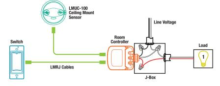
Plug DLM local network components together in any configuration using Cat 5e cables with RJ45 connectors.
