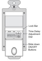
To access adjustment dial, gently pull the lock bar away from the switch face and slide the on/off button down.
