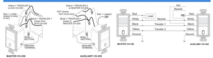
For single pole applications, cap off the yellow wire. Up to four multi-location sensors may be connected together. For details on connecting RH-253s for multi-location control, see the RH-253 cutsheet.
