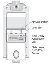
To access adjustment dial, gently pull the lock bar away from the switch face and slide the on/off button down.
