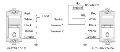
Up to four multi-location sensors may be connected together. For details on connecting RH-253s for multi-location control, see the RH-253 cut sheet.
