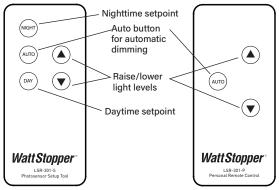
Remote handheld (left) enables easy set-up while optional occupant remote provides adjustability for individual lighting preferences.
