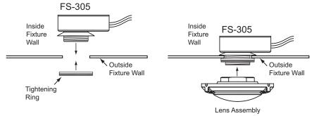
Fig 1: FS-305 mounting in light fixture
