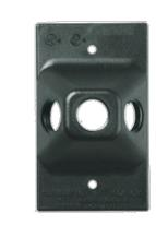
Rectangular cover with three 1/2" threaded holes. Fits FS, cast and recessed single outlet boxes. Supplied with thick foam rubber gasket. One molded 1/2" close-up plug and (2) stainless steel screws.
