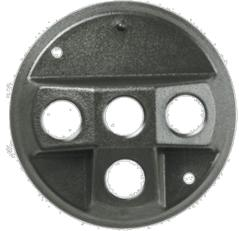
Corrosionproof round four hole cover. Tough polycarbonate with molded-in color. Fourth hole is perfect for motion sensor mounting. Fits 4" round boxes. Supplied with thick foam rubber
