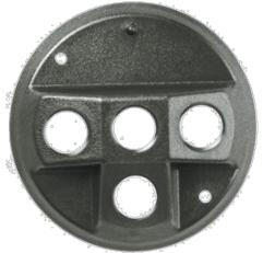
Corrosionproof round four hole cover. Tough polycarbonate with molded-in color. Fourth hole is perfect for motion sensor mounting. Fits 4" round boxes. Supplied with thick foam rubber gasket. One molded 1/2" close-up plug and (2) stainless steel screws.
