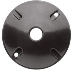
Die cast round covers with one or three 1/2" holes. Fit 4" round boxes. Supplied with thick foam rubber gasket and two #10-24 stainless steel screws. 3 hole cover comes with one die cast 1/2" close-up plug.
