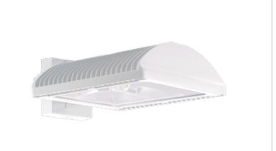
Type: Constant Current Watts: 105W 120V: Color Temp: 3000K (Warm) 208V: 0.58A 81 CRI Color Accuracy: 240V: 0.50A L70 Lifespan: 100,000 277V: 0.44A Lumens: 8,461 Input Watts: 106W Efficacy: 80 LPW Efficiency: 99%
