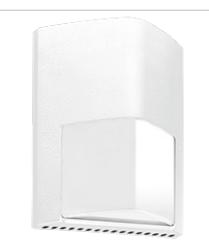
Affordable, high-performance, low-maintenance LED doorway light. Suitable for mounting heights up to 10', and replaces 70W high pressure sodium. 100,000-Hour LED lifespan. 5-Year warranty.
