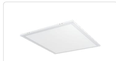
2' x 2' EZPAN edgelit LED panel lights with emergency battery Backup that will operate the LED Lamp for 90 minutes if power fails. For use in drop ceilings or drywall using the optional recessed mounting kit.
