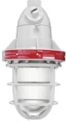
Explosionproof fixture for ceiling mounting. Set screw to stern prevents rotation. Cast aluminum housing, heat and impact resistant globe. Fits all incandescent lamps up to 300 Watt PS-25. Lamp not supplied.
