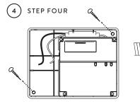
Mount the Gateway to the installation surface using size 10 screws appropriate for the surface material. For direct installation onto an external junction box, use the junction box's included screws.
