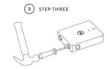
Remove a knockout (KO) from the Gateway using a flat-blade screwdriver and hammer. Place the screwdriver blade at the edge of the KO, then tap the screwdriver with the hammer to weaken the attachment. Work your way around the edge of the KO until it breaks away.
