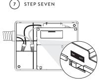
Turn on the Gateway main power switch. Replace outer cover and use included screws to secure.
