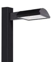
Project: Type: Prepared By: Date: **Driver Info** LED Info Constant Current Watts: 150W Type: 120V: 1.31A Color Temp: 3000K (Warm) 208V. 0.80A Color Accuracy: 81 CRI 240\/-0.69A 100.000 L70 Lifespan: 277V: 0.60A Lumens: 11,352 Input Watts: 153W Efficacy: 74 LPW
