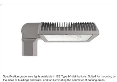
Project: Type: Prepared By: Date: LED Info **Driver Info** Type: Constant Current Watts: 150W 120V: 1.31A Color Temp: 3000K (Warm) 208V: N/A Color Accuracy: 81 CRI 240V: N/A L70 Lifespan: 100,000 277V: N/A 11,352 Lumens: Input Watts: 153W Efficacy: 74 LPW Efficiency: 98%
