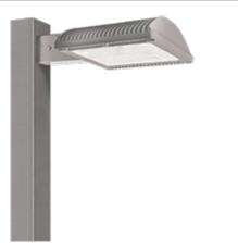
Project: Type: Prepared By: Date: **Driver Info** LED Info Constant Current Watts: 150W Type: 120V: 1.31A Color Temp: 4000K (Neutral) 208V. 0.80A Color Accuracy: 82 CRI 240\/-0.69A L70 Lifespan: 100,000 277V: 0.60A Lumens: 11,786
