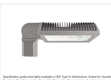
Project: Type: Prepared By: Date: LED Info **Driver Info** Type: Constant Current Watts: 125W 120V: 1.12A Color Temp: 3000K (Warm) 208V: N/A Color Accuracy: 81 CRI 240V: N/A L70 Lifespan: 100,000 277V: N/A 10,464 Lumens: Input Watts: 136W Efficacy: 77 LPW Efficiency: 92%
