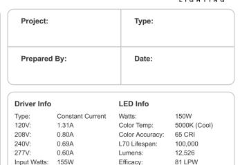
Specification grade area lights available in IES Type III distributions. For use for roadway, general parking and other area lighting applications where a larger pool of lighting is required. Replaces up to 400W metal halide. Patent pending thermal management system. 5 Year Warranty.
