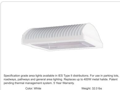
Project: Type: Prepared By: Date: LED Info **Driver Info** Type: Constant Current Watts: 150W 120V: 1.31A Color Temp: 3000K (Warm) 208V: 0.80A Color Accuracy: 81 CRI 240V: L70 Lifespan: 0.69A 100,000 277V: 0.60A 11,494 Lumens: Input Watts: 156W Efficacy: 74 LPW Efficiency: 96%
