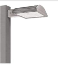
Project: Type: Prepared By: Date: **Driver Info** LED Info Constant Current Watts: 150W Type: 120V: 1.31A Color Temp: 3000K (Warm) 208V. N/A Color Accuracy: 81 CRI 240\/-N/A L70 Lifespan: 100,000 277V: N/A Lumens: 11.576
