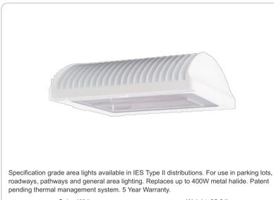
Project: Type: Prepared By: Date: **Driver Info** LED Info Type: Constant Current Watts: 125W 120V: 1.12A Color Temp: 3000K (Warm) 208V: 82 CRI 0.70A Color Accuracy: 240V: 0.61A L70 Lifespan: 100,000 277V: 0.52A Lumens: 10,505 Input Watts: 138W Efficacy: 76 LPW Efficiency: 91%
