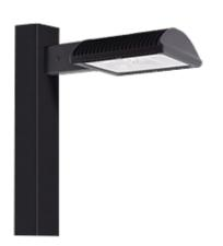
Specification Grade Area lights available in IES Type IV distributions. For use in parking lots, roadways, pathways and general area lighting. Mounts to 4" square steel poles at 15-25'. Designed to replace 250W Metal Halide Area Lights. Patent Pending thermal management system. 5 Year Warranty.
