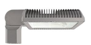
Specification Grade Area lights available in IES Type IV distributions. For use in parking lots, roadways, pathways and general area lighting. Mounts to 4" square steel poles at 15-25'. Designed to replace 250W Metal Halide Area Lights. Patent Pending thermal management system. 5 Year Warranty.
