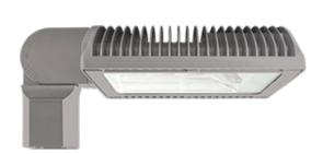
Specification Grade Area lights available in IES Type IV distributions. For use in parking lots, roadways, pathways and general area lighting. Mounts to 4" square steel poles at 15-25'. Designed to replace 250W Metal Halide Area Lights. Patent Pending thermal management system. 5 Year Warranty.
