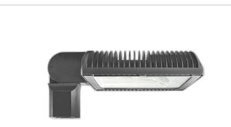
Specification Grade Area lights available in IES Type IV distributions. For use in parking lots, roadways, pathways and general area lighting. Mounts to 4" square steel poles at 15-25'. Designed to replace 250W Metal Halide Area Lights. Patent Pending thermal management system. 5 Year Warranty.
