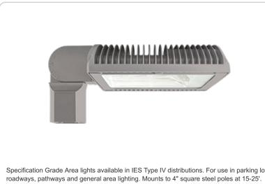
Specification Grade Area lights available in IES Type IV distributions. For use in parking lots, roadways, pathways and general area lighting. Mounts to 4" square steel poles at 15-25'. Designed to replace 250W Metal Halide Area Lights. Patent Pending thermal management system. 5 Year Warranty.
