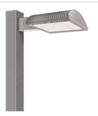
Specification Grade Area lights available in IES Type IV distributions. For use in parking lots, roadways, pathways and general area lighting. Mounts to 4" square steel poles at 15-25'. Designed to replace 250W Metal Halide Area Lights. Patent Pending thermal management system. 5 Year Warranty.
