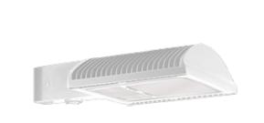
Specification Grade Area lights with multi-level motion sensor available in IES Type IV distributions. For use in parking lots, roadways, pathways and general area lighting. Mounts to 4" square steel poles at 15-25'. Designed to replace 250W Metal Halide Area Lights. Patent Pending thermal management system. 5 Year Warranty.
