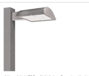
Specification Grade Area lights available in IES Type IV distributions. For use in parking lots, roadways, pathways and general area lighting. Mounts to 4" square steel poles at 15-25'. Designed to replace 250W Metal Halide Area Lights. Patent Pending thermal management system. 5 Year Warranty.
