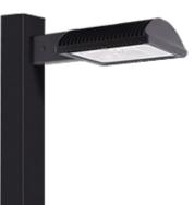
Specification Grade Area lights available in IES Type IV distributions. For use in parking lots, roadways, pathways and general area lighting. Mounts to 4" square steel poles at 15-25' Designed to replace 250W Metal Halide Area Lights. Patent Pending thermal management system. 5 Year Warranty.
