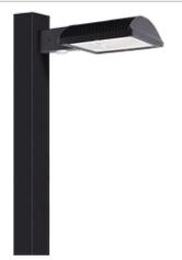
Specification Grade Area lights with multi-level motion sensor available in IES Type IV distributions. For use in parking lots, roadways, pathways and general area lighting. Mounts to 4" square steel poles at 15-25'. Designed to replace 250W Metal Halide Area Lights. Patent Pending thermal management system. 5 Year Warranty.
