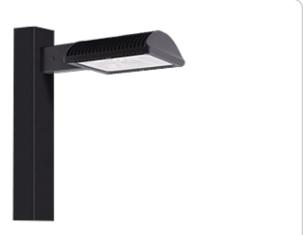
Specification Grade Area lights available in IES Type IV distributions. For use in parking lots, roadways, pathways and general area lighting. Mounts to 4" square steel poles at 15-25'. Designed to replace 250W Metal Halide Area Lights. Patent Pending thermal management system. 5 Year Warranty.
