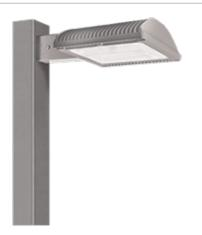
Specification Grade Area lights available in IES Type III distributions. For use in parking lots, roadways, pathways and general area lighting. Mounts to 4" square steel poles at 15-25'. Designed to replace 250W Metal Halide Area Lights. Patent Pending thermal management system. 5 Year Warranty.
