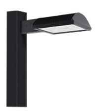
Specification Grade Area lights available in IES Type III distributions. For use in parking lots, roadways, pathways and general area lighting. Mounts to 4" square steel poles at 15-25'. Designed to replace 250W Metal Halide Area Lights. Patent Pending thermal management system. 5 Year Warranty.
