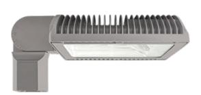
Specification Grade Area lights available in IES Type III distributions. For use in parking lots, roadways, pathways and general area lighting. Mounts to 4" square steel poles at 15-25'. Designed to replace 250W Metal Halide Area Lights. Patent Pending thermal management system. 5 Year Warranty.
