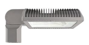
Specification Grade Area lights available in IES Type III distributions. For use in parking lots, roadways, pathways and general area lighting. Mounts to 4" square steel poles at 15-25'. Designed to replace 250W Metal Halide Area Lights. Patent Pending thermal management system. 5 Year Warranty.
