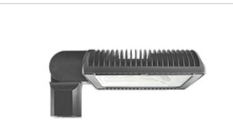
Specification Grade Area lights available in IES Type III distributions. For use in parking lots, roadways, pathways and general area lighting. Mounts to 4" square steel poles at 15-25' Designed to replace 250W Metal Halide Area Lights. Patent Pending thermal management system. 5 Year Warranty.
