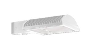
Specification Grade Area lights with multi-level motion sensor available in IES Type III distributions. For use in parking lots, roadways, pathways and general area lighting. Mounts to 4" square steel poles at 15-25'. Designed to replace 250W Metal Halide Area Lights. Patent Pending thermal management system. 5 Year Warranty.
