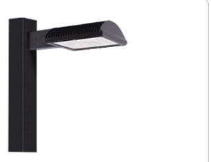
Specification Grade Area lights available in IES Type III distributions. For use in parking lots, roadways, pathways and general area lighting. Mounts to 4" square steel poles at 15-25'. Designed to replace 250W Metal Halide Area Lights. Patent Pending thermal management system. 5 Year Warranty.
