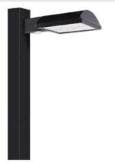
Specification Grade Area lights with multi-level motion sensor available in IES Type III distributions. For use in parking lots, roadways, pathways and general area lighting. Mounts to 4" square steel poles at 15-25'. Designed to replace 250W Metal Halide Area Lights. Patent Pending thermal management system. 5 Year Warranty.
