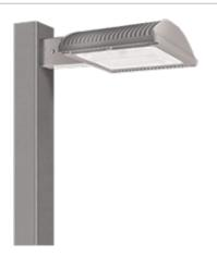
Specification Grade Area lights available in IES Type II distributions. For use in parking lots, roadways, pathways and general area lighting. Mounts to 4" square steel poles at 15-25'. Designed to replace 250W Metal Halide Area Lights. Patent Pending thermal management system. 5 Year Warranty.
