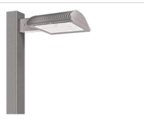
Specification Grade Area lights available in IES Type II distributions. For use in parking lots, roadways, pathways and general area lighting. Mounts to 4" square steel poles at 15-25". Designed to replace 250W Metal Halide Area Lights. Patent Pending thermal management system. 5 Year Warranty.
