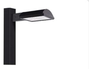
Specification Grade Area lights available in IES Type II distributions. For use in parking lots, roadways, pathways and general area lighting. Mounts to 4" square steel poles at 15-25". Designed to replace 250W Metal Halide Area Lights. Patent Pending thermal management system. 5 Year Warranty.
