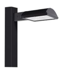
Specification Grade Area lights available in IES Type II distributions. For use in parking lots, roadways, pathways and general area lighting. Mounts to 4" square steel poles at 15-25'. Designed to replace 250W Metal Halide Area Lights. Patent Pending thermal management system. 5 Year Warranty.
